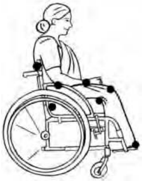
Fig. 2.5. Common pressure sensitive areas (side view)
